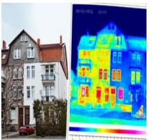
Thermic image of a building which has only partly been insulated © Ingo Bartussek/Adobe Stock
