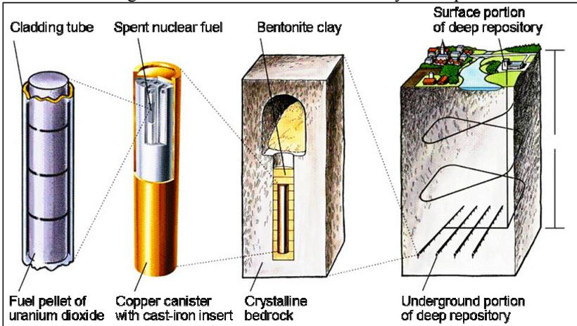
Lastly, the copper canisters are surrounded, when stored, by bentonite clay (5<sup>th</sup> barrier) impervious to water and which immobilises radioelements.
