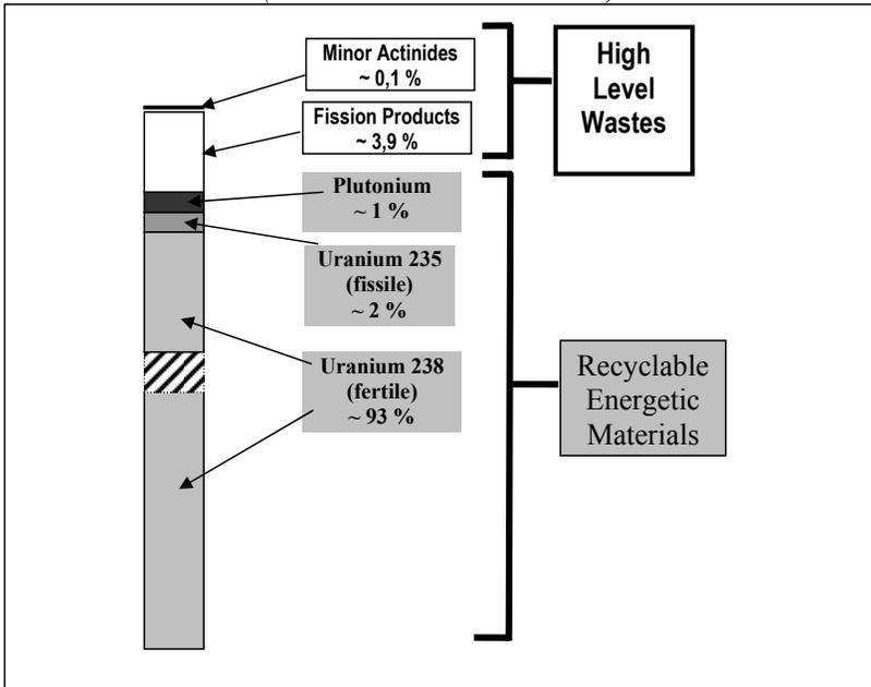
The reprocessing carried out at the La Hague facilities allows uranium and plutonium to be isolated and its main aim is to recover uranium and plutonium, energetic materials, with a view to recycling them. Its second consequence is to reduce the long-term radiotoxicity of wastes.
