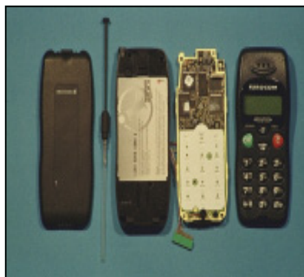
Exploded of a mobile phone - Source : CNRS
