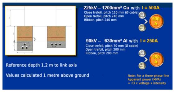
The field produced varies depending on the strength of the current and the configuration of the installation (gaps between the cables):
